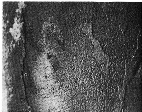
Fig. 3 Surface of the 2.25 percent Cr—1 percent Mo superheater tube from Allen Station after 2400 quench cycles (16X)
